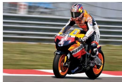
**4.0** **THE NUMBER OF SECONDS** it would take a Grand Prix bike to go from 0 to 62 m.p.h. and back to 0. Remarkably, G.P. bikes can decelerate more quickly than they accelerate, thanks to huge carbon fiber disc brakes. When braking at maximum power, a rider rises up and uses wind resistance to help slow down, as in the photo of Hayden above.
