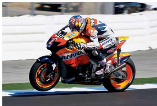
**202** **NICKY HAYDEN’S TOP SPEED**, reached at the Chinese Grand Prix in May. MotoGP bikes, which weigh about 300 pounds and produce more than 220 horsepower, are among the fastest accelerating machines on earth (0 to 62 in 2.1 seconds); at full throttle, their engines rev at more than 18,000 r.p.m.’s.
