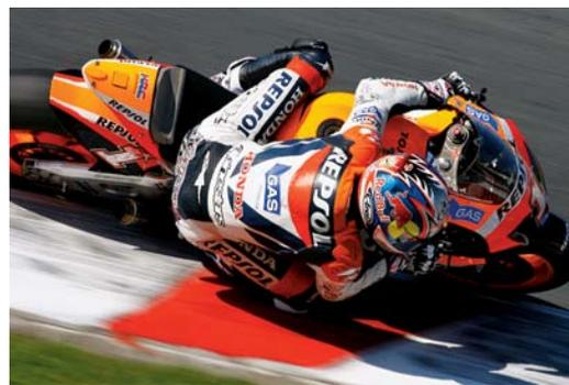
**60+** **THE MAXIMUM LEAN ANGLE** (in degrees) of a rider while he’s cornering. Only a tiny patch of tire rubber (smaller than a credit card) keeps the motorcycle on the road. Hayden’s knees, which actually slide on the pavement in the corners, are covered with hard plastic protectors. By race’s end, they are almost worn through.
